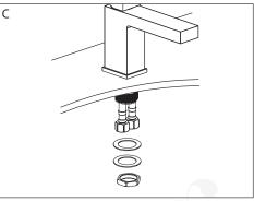
C. Insert the plastic washer, metal washer, and secure the faucet with the mounting nut.
