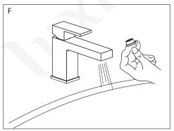
F. Remove the aerator and let the water run for about 1 minute to clear any debris in the plumbing system. Check for leaks at all connections. Reinstall the aerator to complete the installation.
