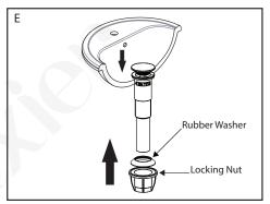
E. Remove rubber washer and locking nut from the drain assembly and slide the drain into the sink. Install the rubber washer first and tighten the locking nut to install the drain.
